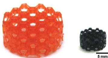
Fig. 1. 3D printed \text{UC}_2/\text{C} nanocomposite as-printed (left) and upon carbothermal reduction (right).
